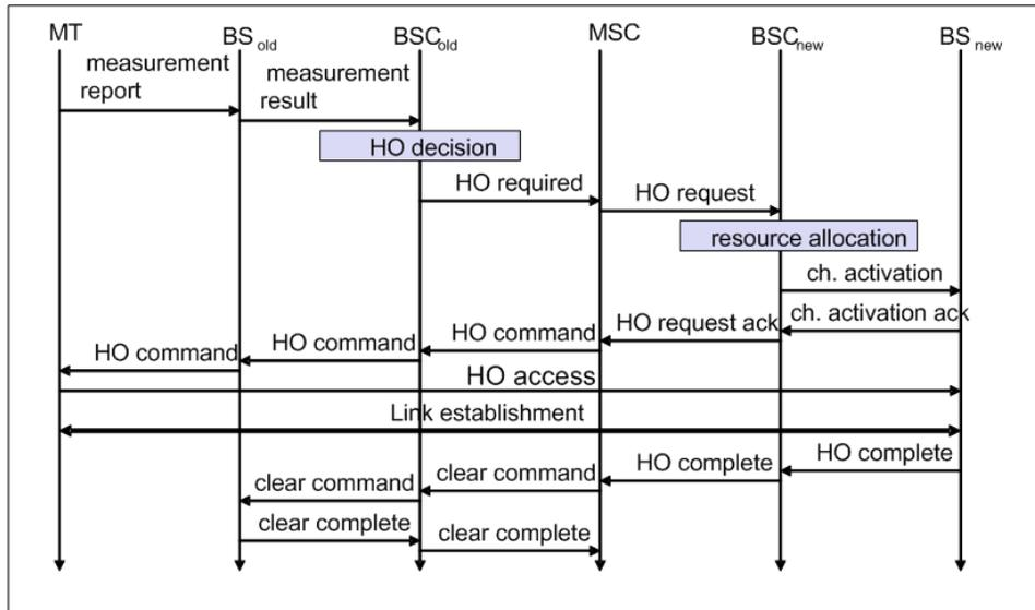
Fig. 1. Hard Handoff Process (redrawn from [8])
