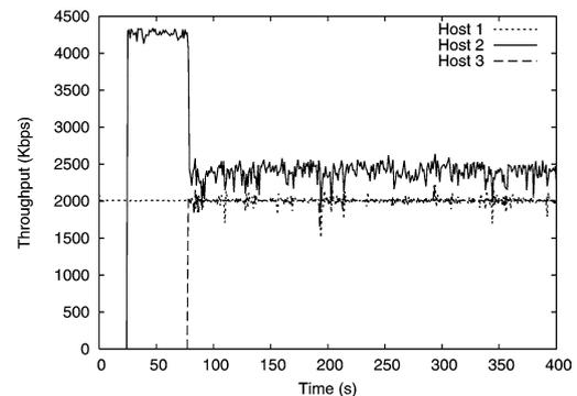
Figure 8. Diffserv over CSMA/CA based hosts.
