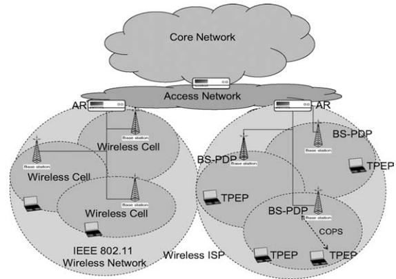
Figure 5. PBM architecture in the wireless network.
