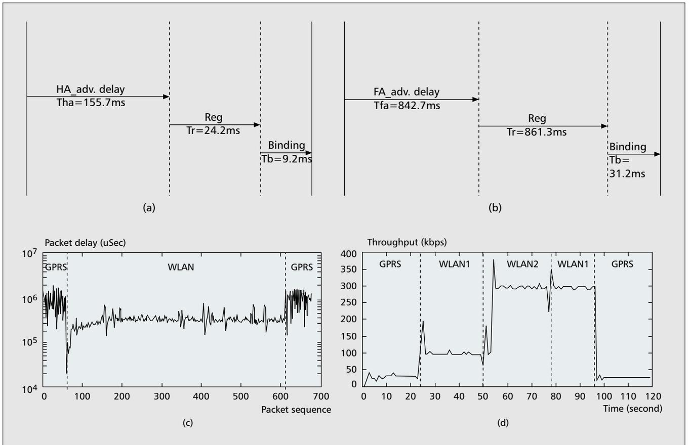
■ **Figure 7.** Experiment results: the home network is in a WLAN (CN: a fixed host outside GPRS): a) handoff latency from GPRS to WLAN; b) handoff latency from WLAN to GPRS; c) TCP packet delay; d) video throughput.
