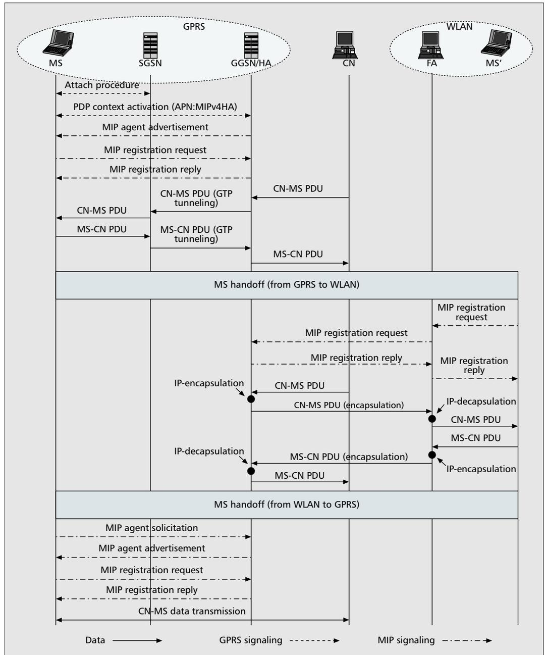
■ **Figure 4.** Intersystem roaming: the home network is in the GPRS.
