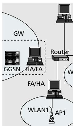
The authors present a gateway approach to the integration of GPRS and wireless LANs (WLANs). The proposed architecture leverages Mobile IP as the mobility management protocol over WLANs.
