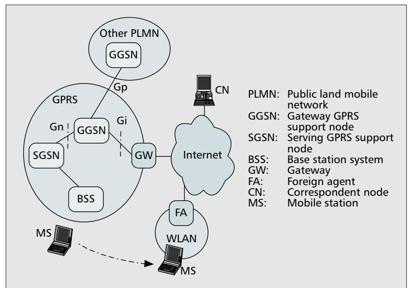
Figure 2. Architecture of the gateway approach.
