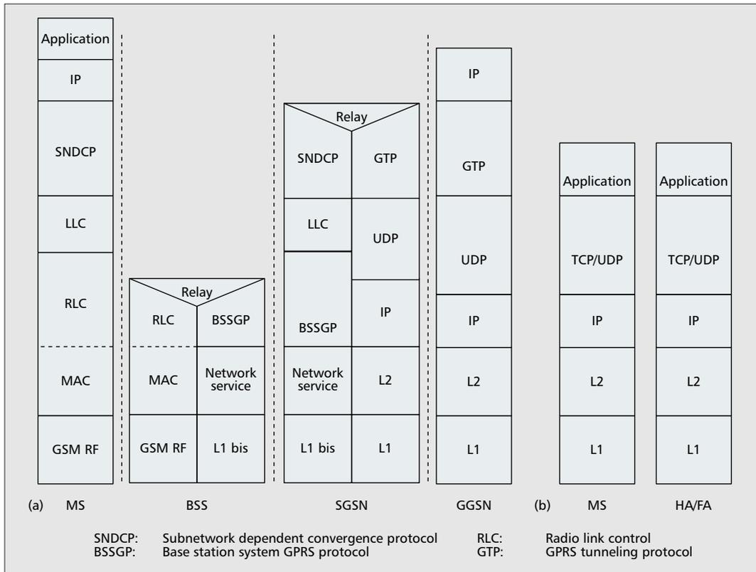
■ **Figure 5.** Dual protocol stacks: a) GPRS user plane; b) IP stack.
