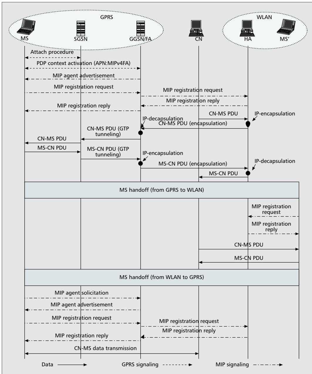
■ **Figure 3.** Intersystem roaming: the home network is in a WLAN.
