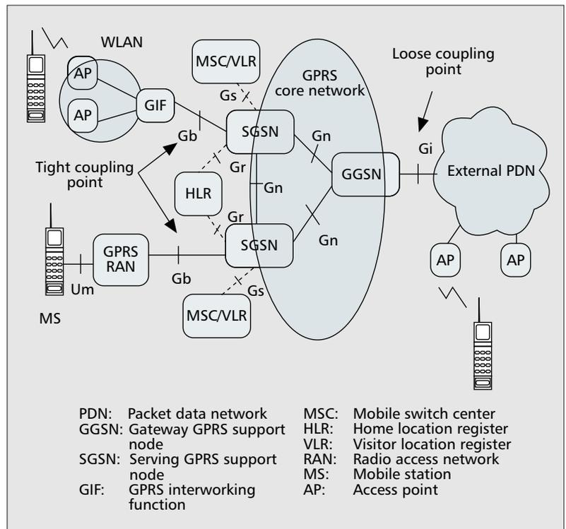
Figure 1. Loose coupling vs. tight coupling.
